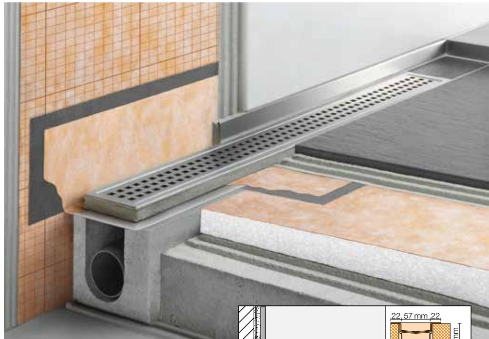
**Schlüter-KERDI-LINE-V 50 G2** for vertical drainage is equipped with an odour trap that is integrated into the drain body. In accordance with DIN 1253, it has a drain capacity of  $\geq 1.0$  l/s (with 20 mm head of water) and a water trap height of 50 mm. Height of channel support:
